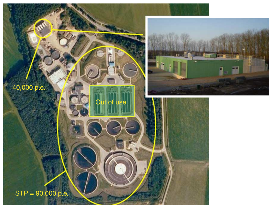
Figure 1 | Reduction of space requirement by separate treatment of industrial wastewater and reject water (upper circle) with a capacity of 40,000 p.e. compared to the sewage treatment plant with a capacity of 90,000 p.e.; picture of the separate treatment in frame.
