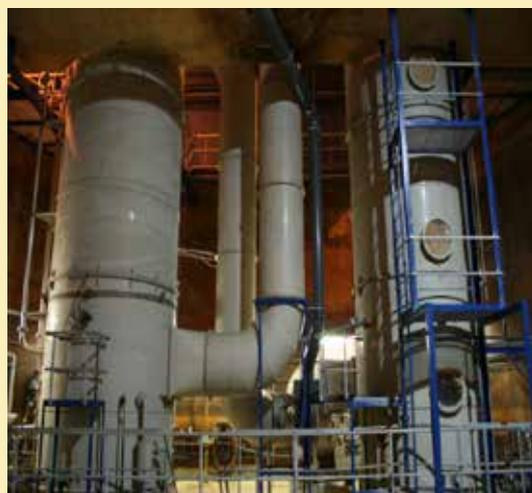
**Picture (Courtesy of VEAS).** Nitrogen recovery at VEAS wastewater treatment plant in Oslo (Norway). Right is the ammonia stripping tower, and left the acid absorption tower.
